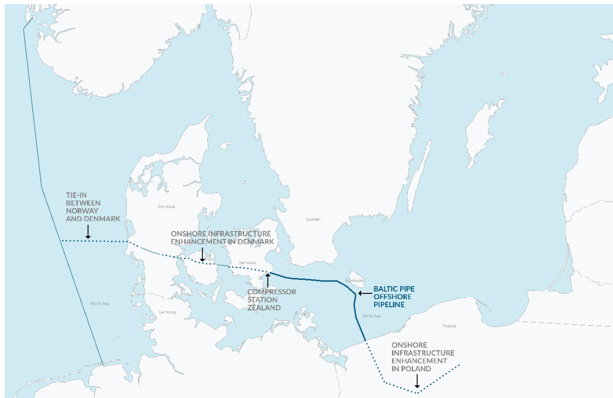
Figure 1-1 Schematic representation of the five major components of the Baltic Pipe project.
