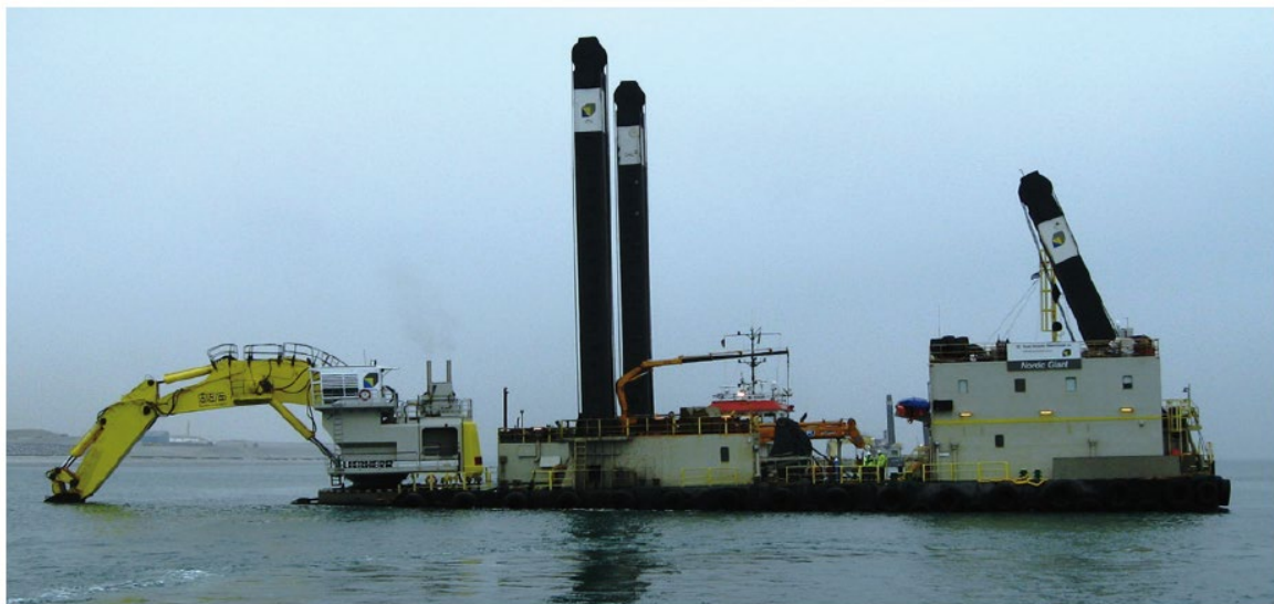
Figure 3-8 Typical backhoe dredge for trenching in shallow water.
